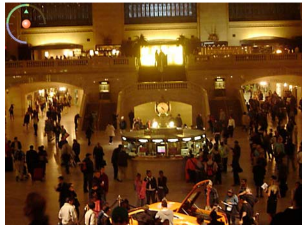
Fig 9. Loudness meter superimposed onto a TV picture. The outer ring shows short-term loudness, the arrow shows long-term loudness. For both indicators, 12 o' clock represents Reference loudness. The red center indicator would normally be off. It signifies notable channel differences, and electrical low or high level.
